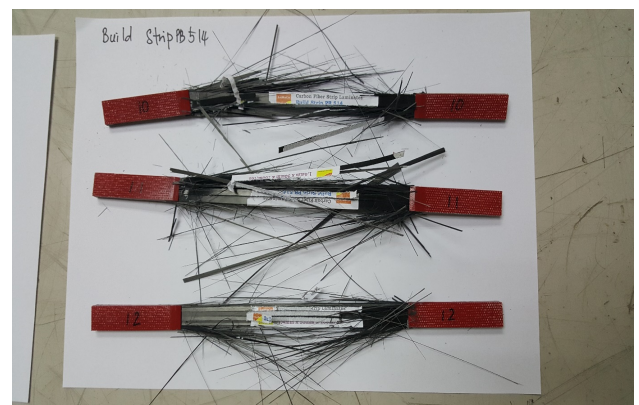
Specimen Samples: [Tested] CFRP Strip 1.4mm x 10mm x 250mm
