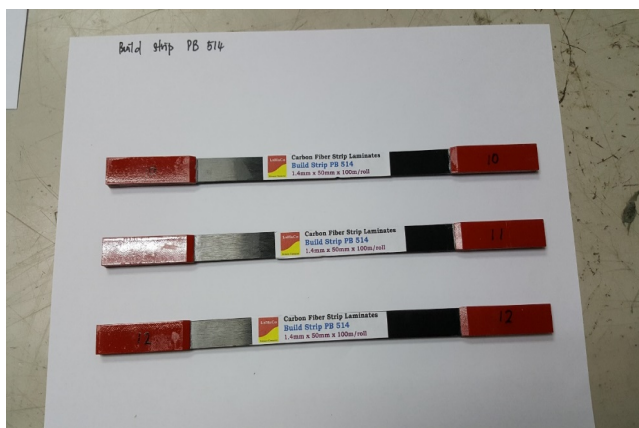
Specimen Sample: [Before Testing] CFRP Strip 1.4mm x 10mm x 250mm
