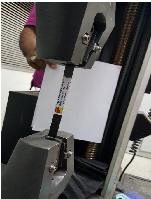
Specimen Sample: [Before Testing] CFRP Strip 1.4mm x 10mm x 250mm
