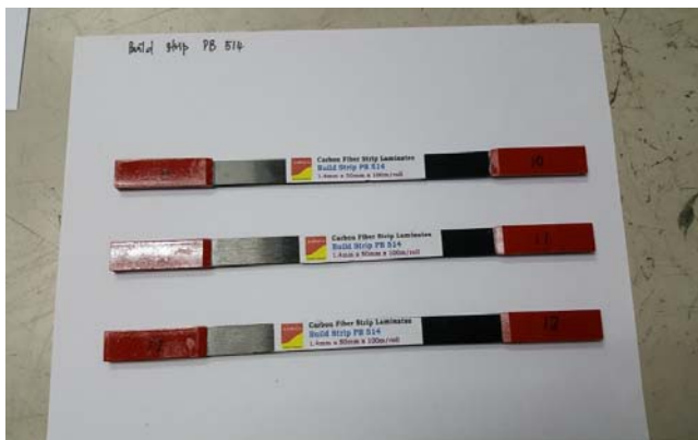
Specimen Sample: [Before Testing] CFRP Strip 1.4mm x 10mm x 250mm
