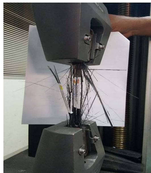
Testing Equipment, Method of Tester Installed, Once Tested the CFRP Cured Laminates Breaking
