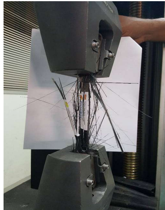
Testing Equipment, Method of Tester Installed, Once Tested the CFRP Cured Laminates Breaking
